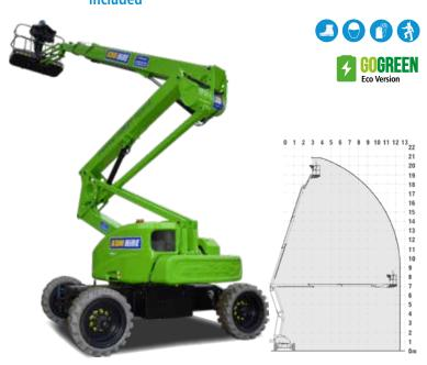
The Nifty HR21 Hybrid Boom offers all the features of our standard 20m Articulating Boom Lifts but provides a more compact and lightweight option for those confined or weight sensitive areas. The hybrid feature allows all electric, noise and fume free operation with the option to switch to engine for outdoor use when battery levels are low. This machine also offers an additional 1m of outreach and exceptional outside turning radius of only 3.89m.
