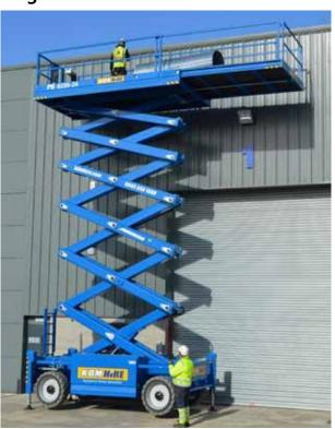
With a massive maximum working height of 22.5m and lift capacity of 1,000kg this heavy duty Diesel Scissor Lift is ideal for large industrial or construction applications.
