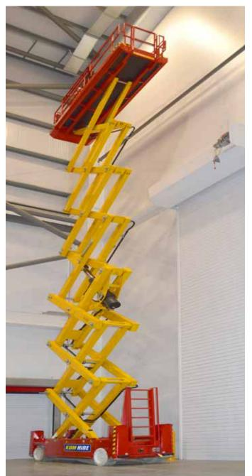
These impressive Scissor Lifts provide a maximum working height of 19m or 22.5m (depending on the model) while still only 1.22m wide. An automatic levelling system provides the user with additional stability allowing indoor or outdoor use. Ideal for high level narrow warehouse aisle applications or inner-city applications on narrow pathways etc.
