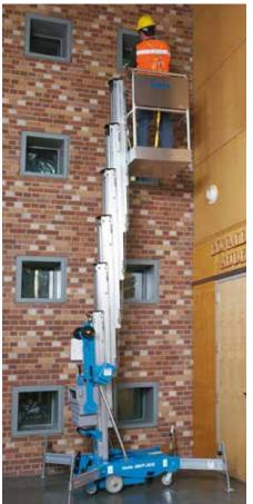
These lightweight vertical lifts can be wheeled through a single doorway allowing work to be safely completed.
