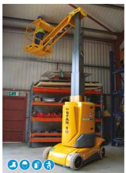
With zero tail swing, a short wheelbase and at only 990mm wide, this machine offers excellent manoeuvrability in confined areas. This Vertical Mast Lift also provides 3.1m of outreach making it ideal for factory maintenance and repair tasks.
