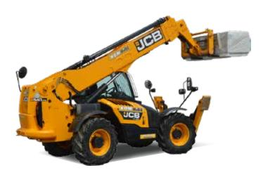
With lift capacities up to 4t and forward reach of up to 13.08m, these 17 & 18m handlers are the ultimate performers around the site. These well balanced machines ensure precision placement of loads. Side shift and frame levelling are available on most models.
