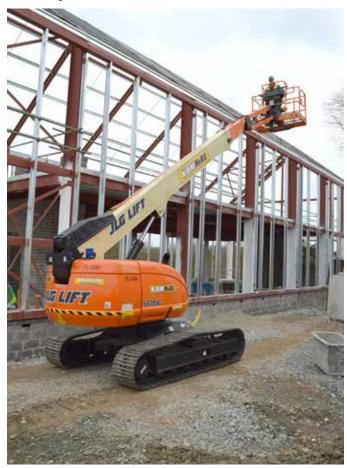
When you need ultimate terrainability, choose this Telescopic Boom Lift. A crawler undercarriage, improved manoeuvrability on soft surfaces and zero turning radius get you to places others just cannot go. Suitable for the most arduous sites and extremely rough terrain. Ideal for transmission line work.
