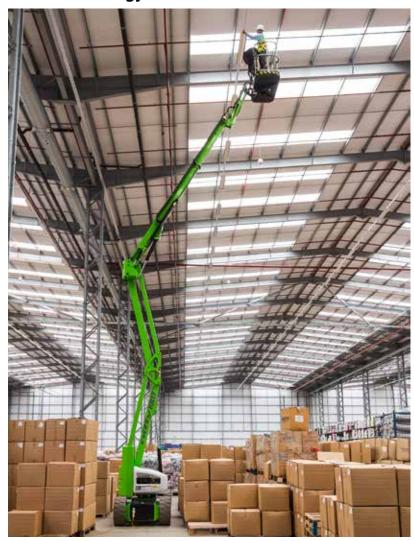
This narrow Self-propelled Boom will lift to a working height of 17.2m and provide an exceptional outreach of 9.7m. 180° platform rotation provides exceptional control when positioning the platform in narrow, confined spaces where there is a need to reach over machinery or fixed objects.
