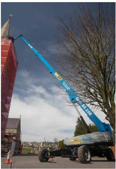
With up to 48m working height and x-chassis design providing extra stability, this Super Boom is ideal for extreme access jobs. It has positive traction drive, a self levelling platform, rough terrain foam filled tyres and an on board generator as standard. A 10' Rotating Jib gives perfect positioning for any task.
