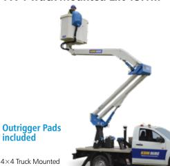
4×4 Truck Mounted Platforms offer a working height of 13.1m and 6.2m outreach ideal for utility, telecom or streetlight maintenance where the task requires quick and easy site set up. 360° rotation, 240kg platform capacity and zero tail swing allowing operators to access the most difficult working areas.
