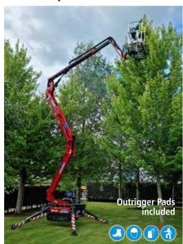
This 17m Spider Lift is ultra compact allowing you to work in the most difficult to access areas. Designed to go just about anywhere including ground sensitive areas where weight or disturbance is a concern. Ideal for tree surgery in parks or a range of maintenance jobs inside or out.
