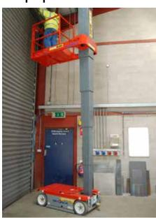
When operating in tight workspaces, a short wheel base and high degree steer angle provide these machines with superior functionality and efficiency over conventional scissor lifts. Slide out deck extensions on most machines also allow up and over capability.
