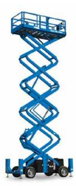
These large twin-decked machines offer exceptional deck space up to heights of 18m, making these Scissors ideal for your largest cladding and roofing applications. Puncture proof tyres and auto-level jacklegs fitted as standard.
