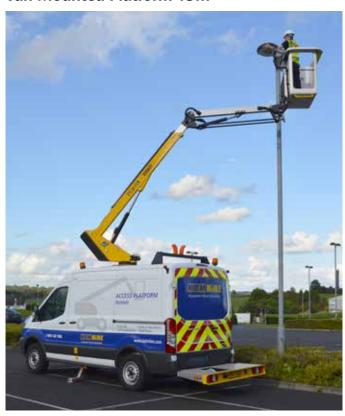
These Van Mounted Platforms are ideal for applications such as street light or sign maintenance where you need additional payload capacity for tools and materials.
