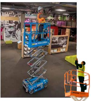
The Genie® GS-1330m scissor lift offers a maximum platform height of 12.8ft (3.9m) and a maximum working height of 18.8ft (5.9m), with a 2-person, 500lb (227kg) capacity and weighing in at only 1950lb (885kg). The Genie GS-1330m scissor lift is equipped with an efficient, all-electric DC drive system that offers productive power for getting around indoor job sites with quiet, zero-emissions operation.
