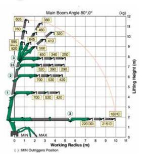
NEW The Innovative Maeda 3053C Knuckle boom crane offers addition versatility, reach, and lift height over other machines. With a 16.95m maximum lift height while still only 780mm wide, this crane will get into areas and lift where others cannot. A three section fully automatic telescopic boom along with stepless outrigger settings provides the up and over versatility and capabilities that other cranes cannot offer.
