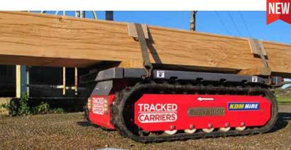
This state of the art tracked mover removes the need for manual handling, reduces labour costs and increases productivity when handling or transporting larger components into tighter spaces. Battery powered with radio remote control, the tracked carrier will handle difficult sites and gradients with ease while keeping the operator a safe distance away. Swivel platform and dolly accessory options are available to make long load handling safe and simple.
