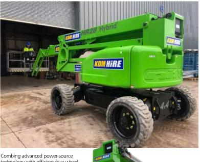
technology with efficient four-wheel drive allow this 28m articulating boom to work in any environment, indoors or out. Emission free operation and reduced running costs along with a lighter weight and more compact foot print make this one of the versatile boom lifts available.
