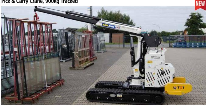
The unique tracked pick and carry crane allows safe positioning and handling of goods or materials on soft ground or rough terrain. The tracked crawler chassis provides low ground pressures while retractable tracks allow access to narrow driveways or paths. With a lift capacity of 900kg, forward reach of over 3m and lift height of 4.3m, the tracked pick and carry crane is ideal for positioning glass, marble slabs or structural beams in otherwise hard to reach places.
