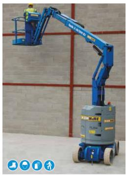
For working in narrow factory aisles or places where larger booms cannot reach. Rotating jib and basket allows perfect work positioning.
