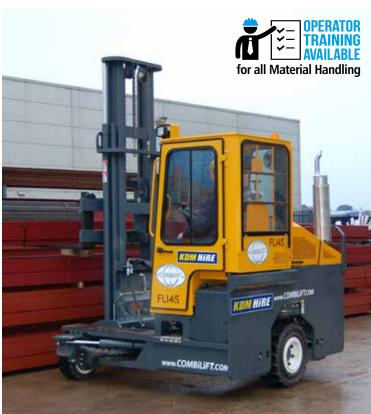
The Combilift encompasses three machines in one - a Counterbalance Forklift, Aisle Truck and Side Loader.
