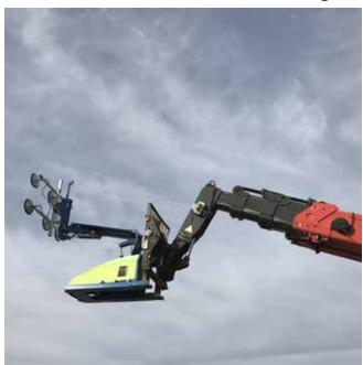
NEW This glass positioner fits directly to the forks of a telehandler or forklift for installation of glass at height or where ground conditions are difficult. With a 350kg capacity and operated by a cabled remote control, the unit allows safe handling and manipulating of glass in places a standard unit cannot reach.
