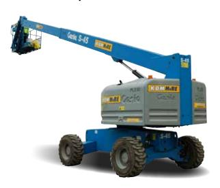
With 4WD and flick-out jibs as standard, these Rugged Telescopic Booms are ideal for a host of applications, including structural steel and general maintenance work.
