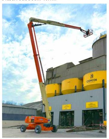
The JLG 1250AJP's unique boom design significantly reduces lift/lower cycle times for the operator while the dual platform capacity of up to 450kg allows increased versatility and productivity. With a massive 19.25m of horizontal outreach, full four wheel drive and four wheel steer, this large articulating boom offers superb mobility and high reach access around the site.
