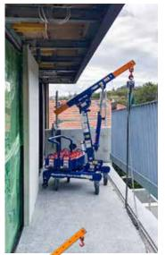
Manual mini floor cranes are designed for lifting applications where no overhead lifting point is available or cannot be accessed by other powered equipment. Easily moved into position these cranes can safely undertake lifts up to 900kg at hook heights of 2.9m. With a maximum outreach of 1.4m floor cranes are particularly advantageous when obstacles or limited floor loadings prevent direct access or the use of forklift.
