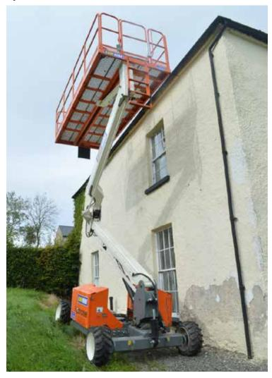
The unique SL30SL Speed Level offers automatic powered platform levelling without the need for outriggers. Level up to 13° from side-to-side and up to 9° from front-to-back swiftly for a stable working platform. Driveable at full height (11m), the Speed Level offers a spacious platform (1.72m x 4.32m) and a powerful 4-wheel-drive ideal for cladding and glazing applications on rough terrain sites even on compound slopes.
