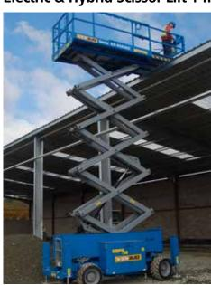
Available in electric hybrid options, these machines provides excellent rough terrain capability whilst offering zero emissions and quiet operation for noise sensitive environments. Other features include a maximum working height of 14.2m and a 4.31m extended deck size.
