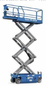
With working heights up to 10m and only 810mm wide, these Narrow Scissors are perfect for manoeuvring into awkward areas. Non-marking tyres allow travel over sensitive floors.
