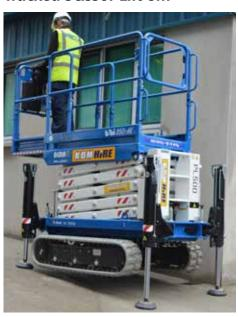
This Tracked Scissor Lift has auto levelling outriggers which extend to 400mm allowing levelling on the most uneven surfaces. Retractable outriggers allow travel through narrow entrances only 800mm wide making this machine ultra versatile.
