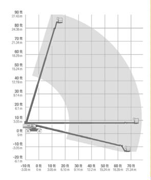
With working heights of up to 28.21m these heavy weight Telescopic Booms are the ultimate in reach and stability. With a dual basket capacity system of 227kg on full reach and 341kg on restricted reach, they have a greater lift capacity than their rivals (\*some models only). Features include full time four wheel drive and fixed width axles (some models only).
