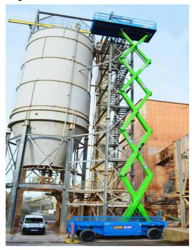
This mega HL-275 D25 Diesel Scissor Lift offers a working height of 27.5m, a working area of up to  $8.25 \, \text{m} \times 2.35 \, \text{m}$  (extended) and a safe working capacity of 1000kg.
