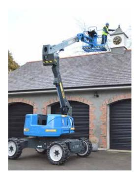
These Booms offer 4WD capability for applications up to 12.6m. With zero tail & nose swing and at only 1.99m wide, these Diesel Booms are ideal for working in confined areas.
