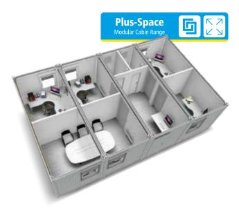
The CS modular building range is a highly flexible building system that allows an infinite number of possibilities and configurations including large site offices, class rooms, laboratory's or show rooms. Standard modules are 6m x 2.4m with a fully flexible wall system that allows windows and doors to be positioned to suit your requirements.
