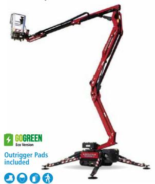
These Tracked Lifts will travel across soft or uneven ground and allow access through narrow gateways or into confined sites. Excellent outreach makes these machines ideal for tree pruning, shopping mall maintenance or work around the house or garden.
