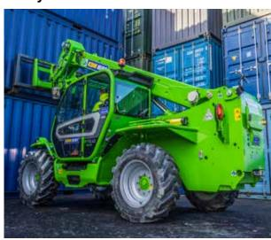
These Heavy Lift Telehandlers are the ultimate site workhorse providing up to 7200kg lifting capacity - 4000kg at full height (9.55m). Ideally suited for safely handling larger heavy loads or large volume shovelling applications.
