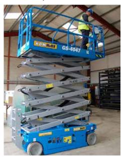
At only 1.19m/3'11" wide and offering a working height of nearly 14m, this Scissor Lift is ideal for high-level maintenance or fit-out of warehouses or factories. A lifting capacity of up to 350kg and a 91cm slide out deck extension make this machine exceptionally versatile. Standard features include solid non marking tyres and folding handrails.
