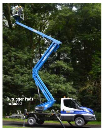
Ideal if your work involves moving from site to site or you need to vacate the site on completion of your task. Vertical outriggers allow quicker set-up on site and less roadside disruption due to their extremely compact footprint.
