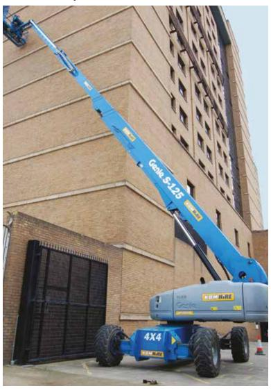
The Genie S125 provides working heights of up to 40.2m and maximum horizontal reach to an impressive 24.4m. Four-wheel drive and four-wheel steer are standard to meet the demands of rugged outdoor use.
