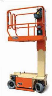
Hydraulically operated vertical mast provides an exceptionally smooth operation while clean and quiet for a variety of environments. Front wheel drive provides outstanding manoeuvrability and long cycle duties.
