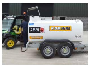
When transporting bulk fuel to site, these Tandem Axle Fuel Bowsers allow you to do so in a safe, legal manner. This Fuel Bowser is fully bunded and compliant with all road towing regulations. Can be used for refuelling or connection to static equipment.
