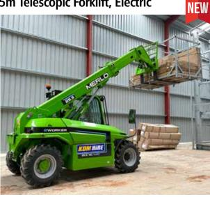
Eliminate polluting emissions and fumes, reduced noise levels, and drastically reducing operating costs, are only some of the compelling reasons to switch to using an electric telehandler. With increased manoeuvrability in confined spaces this is the ideal tool for applications in closed environments such as stables, warehouses, industry or underground environments.
