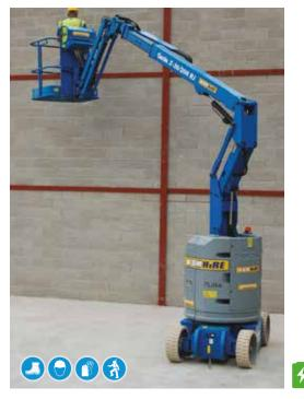
For working in narrow factory aisles or places where larger booms cannot reach. Rotating jib and basket allows perfect work positioning.
