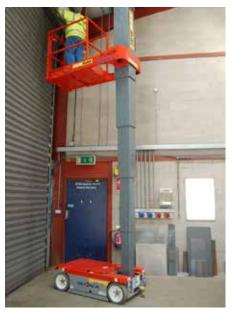
When operating in tight workspaces, a short wheel base and high degree steer angle provide these machines with superior functionality and efficiency over conventional scissor lifts. Slide out deck extensions on most machines also allow up and over capability.
