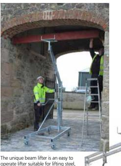
operate lifter suitable for lifting steel, wood beams or other materials into position. Lifts up to 600kg to heights of 3m but will fold down and fit into most estate cars.
