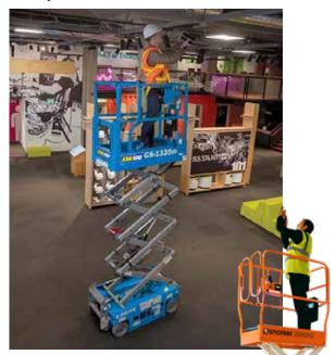
The Genie® GS-1330m scissor lift offers a maximum platform height of 12.8ft (3.9m) and a maximum working height of 18.8ft (5.9m), with a 2-person, 500lb (227kg) capacity and weighing in at only 1950lb (885kg). The Genie GS-1330m scissor lift is equipped with an efficient, all-electric DC drive system that offers productive power for getting around indoor job sites with quiet, zero-emissions operation.
