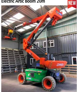
This all electric Boom allows emission free and guiet operation for heights up to 20m. It also boasts the reach characteristics of standard machines but with the advantages of non-marking tyres and continuous 360° rotation while being very economical to run.
