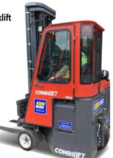
This innovative compact forklift provides the versatility to operate as a narrow aisle forklift, handle long lengths such as steel beams and timber plus still offering the manoeuvrability of a conventional forklift. The low profile and compact design also improves safety and increases productivity. Suitable for indoor and outdoor applications the compact multi directional forklift has the ability to handle a diverse range of goods in most industries.
