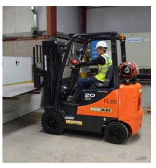
Producing less emissions than conventional diesel forklifts, these Gas Trucks are ideal for use in ventilated warehouses or factories where personnel are working.
