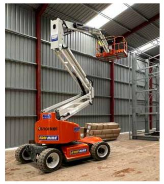
With working heights of up to 15.9m, these guiet, emission-free Lifts can provide outreach capacity of up to 6.1m and full 360° articulation. Perfect for internal jobs, which require high reach and perfect positioning.
