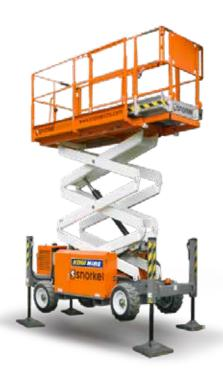
This Narrow diesel scissor lift provides excellent off-road performance but with slim dimensions is still able to access those awkward areas. Ideal for narrow paths or entrances where a conventional machine will not fit. A large deck with roll out extension and self-levelling outriggers make this a versatile workhorse.
