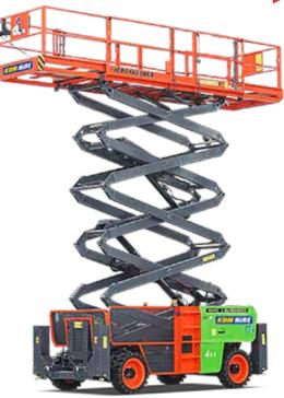
Offering the same features as the standard diesel version but fully electric, these rugged twin deck scissor lifts have an 680kg lift capacity and large 5.41m long deck. Quiet and emission free, this machine will work all day on a single charge.
