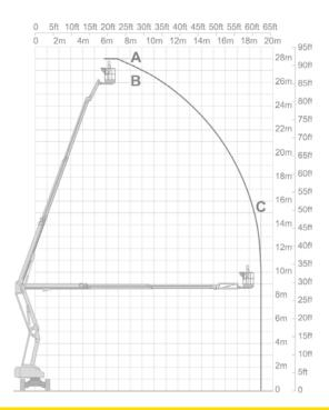
Combining advanced power-source technology with efficient four-wheel drive allow this 28m articulating boom to work in any environment, indoors or out. Emission free operation and reduced running costs along with a lighter weight and more compact foot print make this one of the most versatile boom lifts available.
