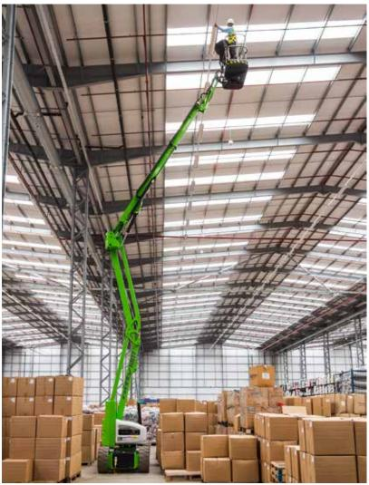
This narrow Self-propelled Boom will lift to a working height of 17.2m and provide an exceptional outreach of 9.7m.  $180^{\circ}$  platform rotation provides exceptional control when positioning the platform in narrow, confined spaces where there is a need to reach over machinery or fixed objects.
