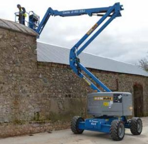
The 45ft Boom is the workhorse of the access industry. 4WD, puncture-proof tyres, zero tail swing and flick-out jibs are just some of the features making this machine perfect for the toughest sites.
