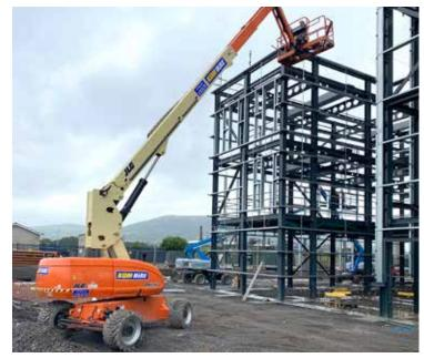
With working heights of up to 28.21m these heavy weight Telescopic Booms are the ultimate in reach and stability. With a dual basket capacity system of 227kg on full reach and 341kg on restricted reach, they have a greater lift capacity than their rivals (\*some models only). Features include full time four wheel drive and fixed width axles (some models only).
