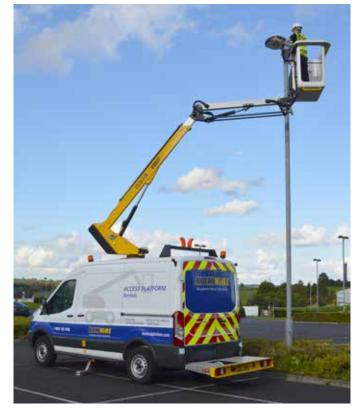
These Van Mounted Platforms are ideal for applications such as street light or sign maintenance where you need additional payload capacity for tools and materials.
