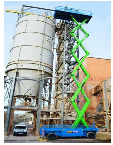
This mega HL-275 D25 Diesel Scissor Lift offers a working height of 27.5m, a working area of up to  $8.25m \times 2.35m$  (extended) and a safe working capacity of 1000kg.
