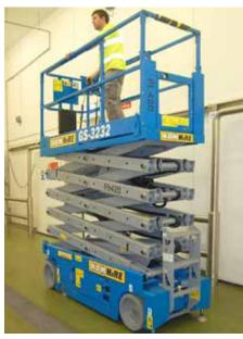
This unique machine has built-in stabilisers to allow work up to an impressive 11.8m whilst still being able to access narrow passageways and aisles.
