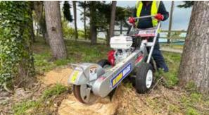
These Petrol driven Stump Grinders provide a safe and easy way to remove stumps without the need to dig or burn.
