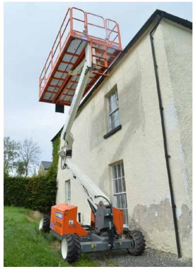
The unique SL3OSL Speed Level offers automatic powered platform levelling without the need for outriggers. Level up to 13° from side-to-side and up to 9° from front-to-back swiftly for a stable working platform. Driveable at full height (11m), the Speed Level offers a spacious platform (1.72m x 4.32m) and a powerful 4-wheel-drive ideal for cladding and glazing applications on rough terrain sites even on compound slopes.
