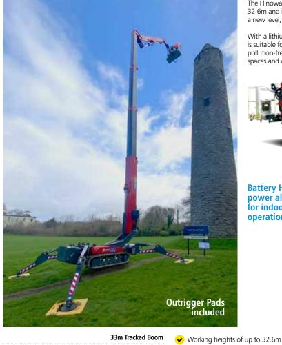
32.6m and is capable of 16.5m outreach, taking up-and-over capabilities to a new level, these impressive booms can also be operated at negative levels. With a lithium battery and diesel engine hybrid power system, this boom is suitable for both indoor and outdoor work offering low noise and pollution-free operation. The compact design allows access to confined spaces and areas other machines simply cannot reach.
