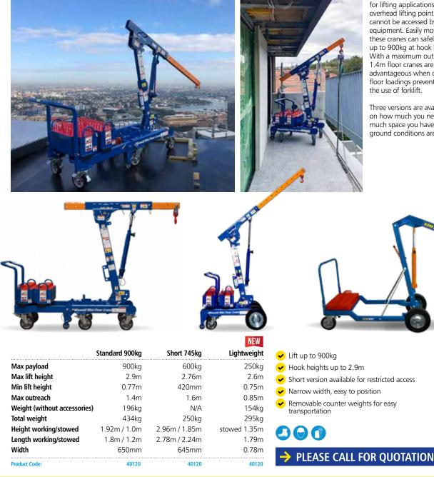
Manual mini floor cranes are designed for lifting applications where no overhead lifting point is available or cannot be accessed by other powered equipment. Easily moved into position, these cranes can safely undertake lifts up to 900kg at hook heights of 2.9m. With a maximum outreach of 1.4m floor cranes are particularly advantageous when obstacles or limited floor loadings prevent direct access or the use of forklift.
