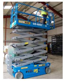
At only 1.19m wide and offering a working height of nearly 14m, this Scissor Lift is ideal for high-level maintenance or fit-out of warehouses or factories. A lifting capacity of up to 350kg and a 91cm slide out deck extension make this machine exceptionally versatile. Standard features include solid non marking tyres and folding handrails.
