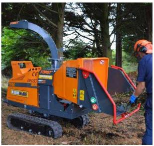
This Tracked Chipper offers the same performance as the towed version but will travel over soft ground or up steep embankments, allowing access to otherwise restricted areas. The tracks can also be extended to provide extra stability on uneven ground.
