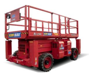
With twin roll-out deck extensions providing a platform size up to 7.38m long and lift capacity of up to 1.1t, these Scissor Lifts will handle the toughest jobs.
