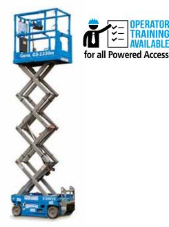
For those hard-to-access areas where turning space is limited, these Compact Scissors are ideal for safe working at heights up to 7.8m. Fold down handrails allow travel through a standard door.
