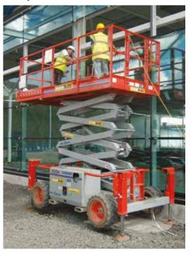
These compact Rough Terrain Scissors will handle the most rigorous sites, but still access those awkward areas. Self-levelling jacklegs provide extra stability and the ability to work on sloped or uneven ground. Standard features include puncture-proof tyres and a roll out deck extension.
