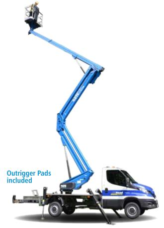
Ideal if your work involves moving from site to site or you need to vacate the site on completion of your task. Vertical outriggers allow quicker set-up on site and less roadside disruption due to their extremely compact footprint.
