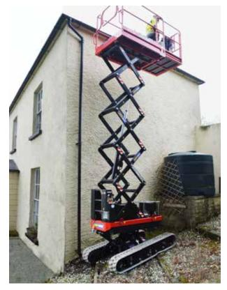
This unique Bi-level Tracked Scissor provides safe access solutions on slopes of up to  $20^{\circ}$ . Capable of levelling both longitudinally and laterally, this machine will operate in the roughest and most uneven conditions. The crawler traction allows access to areas not suitable for traditional  $4 \times 4$  machines.
