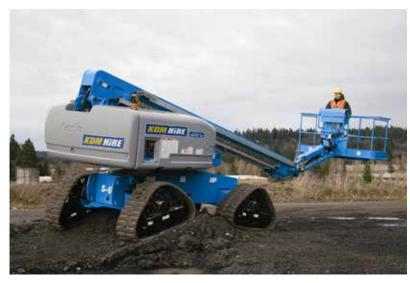
When you need the ultimate in rough terrain ability, the 4-track telescopic boom lift is the only answer. With unique 4-point tracking and oscillating axle this machine offers superior traction allowing it to go where other booms will not. Suitable for the most arduous sites and field conditions, ideal for transmission line work.
