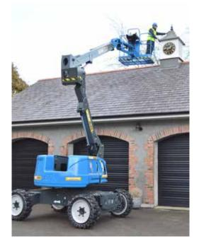
These Booms offer 4WD capability for applications up to 12.6m. With zero tail & nose swing and at only 1.99m wide, these Diesel Booms are ideal for working in confined areas.
