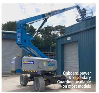
The S60 FE Hybrid boom offers all the capabilities of a standard telescopic boom but with the added benefit of quiet and clean battery operation. The boom is also 25% lighter than a conventional diesel machine making it ideal for city jobs or applications where low floor loading is required.
