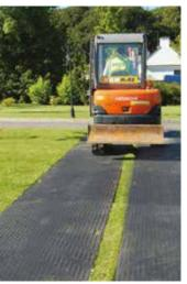
Ground Protection & Pedestrian Mats provide temporary access and ground protection for pedestrian or vehicle movement. These mats are easy to handle with pedestrian mats coloured to demarcate pathways etc. Ground mats can distribute loads of up to 60t and used as roadways or to form parking and turning areas.
