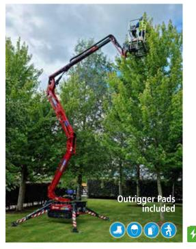
This 17m Spider Lift is ultra compact allowing you to work in the most difficult to access areas. Designed to go just about anywhere including ground sensitive areas where weight or disturbance is a concern. Ideal for tree surgery in parks or a range of maintenance jobs inside or out.
