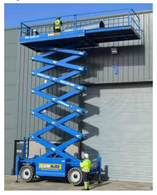
With a massive maximum working height of 22.5m and lift capacity of 1,000kg this heavy duty Diesel Scissor Lift is ideal for large industrial or construction applications.
