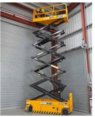
A narrow platform size of 0.81m / 2.64m and a massive 15.8m working height, this scissor is ideal for working at large heights and in tight areas. Fitted with a host of systems including pot hole protection, speed limiting at height and a load sensing system. Standard features include solid non-marking tyres and folding handrails.
