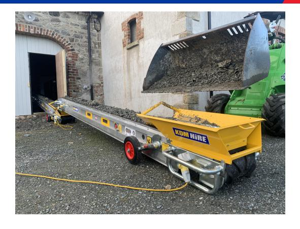
Moving rubble or material to or from your work space couldn't be easier using 4.4m conveyors. The ideal solution when moving large amounts of sand, stone, rubble, soil in the most awkward spaces. All you require is a 110V power connection for a single operator to move up to 60 tonnes per hour at an incline of up to 50 degrees. These machines can also be linked for moving materials over larger distances and around corners.
