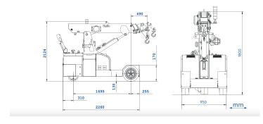
These Mini cranes are designed to operate in confined spaces, capable of a wide range of lifting tacks. With an impressive 2.25 tonne lifting capacity they are still narrow enough to fit through a standard doorway. Suitable for industrial applications where machinery needs moved or for construction sites to carry out glass installations or material lifting tasks where safety and efficiency are essential.
