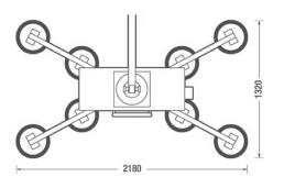
Exceptional slimline design and weighing only 75kg this lifter is ideally suited to working in tight working environments. Capable of lifting up to 750kg with 10 suction cups fitted, this vacuum is an impressive performer.
