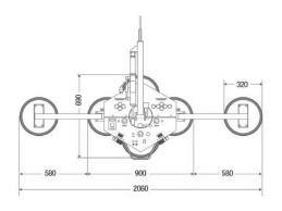
This compact but powerful lifter offers multiple configurations to suit a variety of panel shapes or sizes. The slimline design allows access into the most difficult situations while the variable length extension arms are easy to set up.
