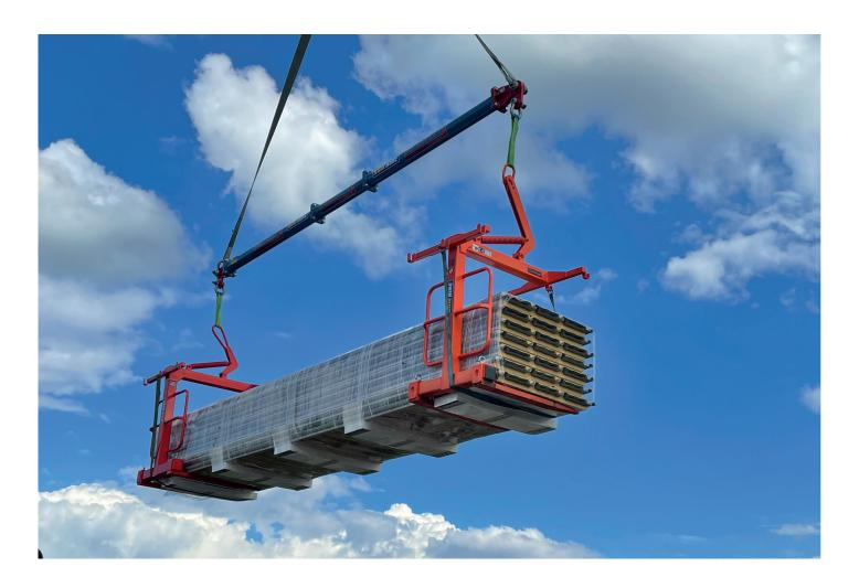
The Bale clad is a simple solution to the lifting and handling of bales of cladding on site. Using a modular spreader beam combined with 2 self-levelling crane forks, bales of cladding can be unloaded and lifted into position quickly and efficiently while avoiding panel damage.
