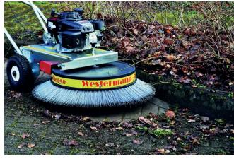
The Westermann WR870 provides a 870mm wire brush head for the easy removal of thick moss from a range of surfaces including block paving, concrete, tarmac or sports surfaces. The clockwise and anti-clockwise rotation of the brush allows you to get into the cracks and crevices where the moss resides, without the use of harsh chemicals or water.
