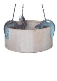
Designed for transporting or laying manhole rings and cones safely.
