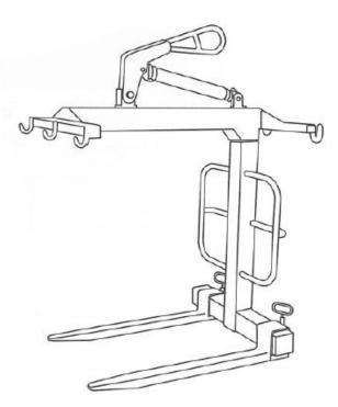
Designed for crane lifting of brick packs and pallets, with adjustable forks. These forks have the advantage of a spring loaded lifting eye which automatically adjusts to compensate for the different weights carried. This ensures that the crane fork stays level, both when empty or full. Fitted with frame to allow attachment of a safety net.
